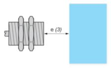
e (3) ≥ 24 mm/0.94 in. Mounted in a metal support
